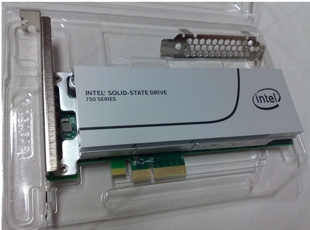
FIGURE 4. A PCIe NVMe SSD
